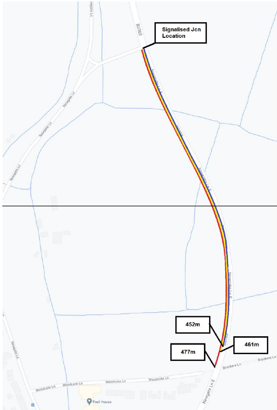
Figure 3: Fully signalised Maximum Queue Length (PCUs) AM peak, HA Modelling Source: Extracted from HA Modelling Fully Signalised, October 2020 (Appendix NG2)
